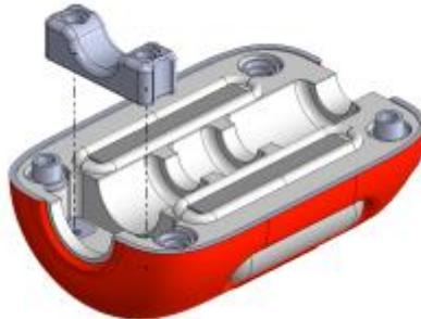
The two-aluminum mounting half-shells ensure that the product is compatible with different cable diameters.
