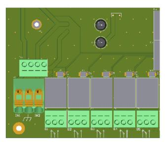
The 48Vdc card has no converter. Each product connected to the board must match the card's voltage rating.
