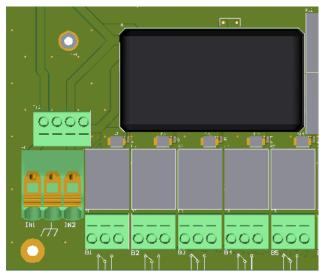
The 240Vac card has an AC/DC converter. Each product connected to the board must match the card's voltage rating.
