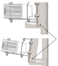
Loosen the two mounting screws to adjust the projector's tilt within a range of 0° to 8°. The bracket has markings every 1° for precise adjustment. Once in position, tighten the nuts to lock the spotlights in place.
