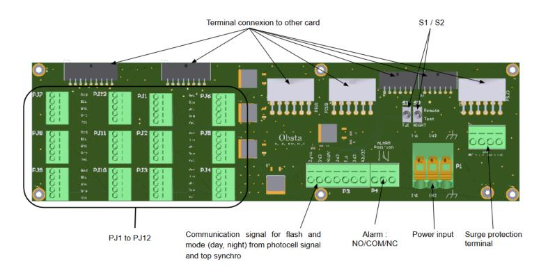
PJ1 to PJ12 / Projector connector must be connected according to the cable color or number. Other harnesses are cabled directly from the factory. Do not modify the cabling without Obsta's direct consent.
