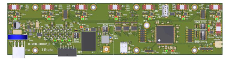
This part is responsible for managing the whole flash head. The embedded microcontroller can analyse input signals (such as GPS, various external signals) and act accordingly.
