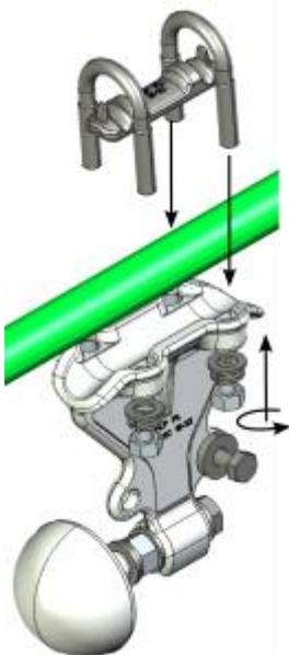
1. Install nuts, clamps and upper jaw.
