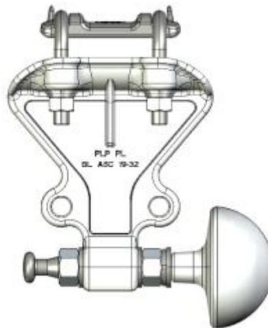
1. Install nuts, clamps and upper jaw.
