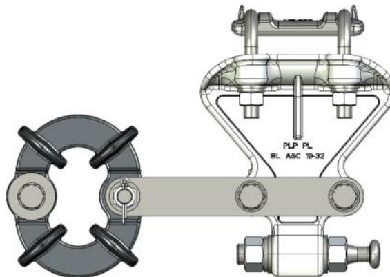
1. Install nuts, clamps and upper jaw.
