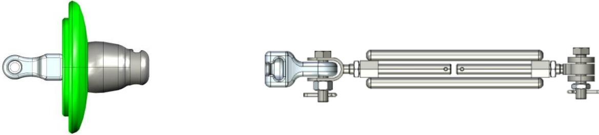
1. Assemble the tensioner on the antenna, tighten all fasteners to 45 Nm and secure them with pins.
