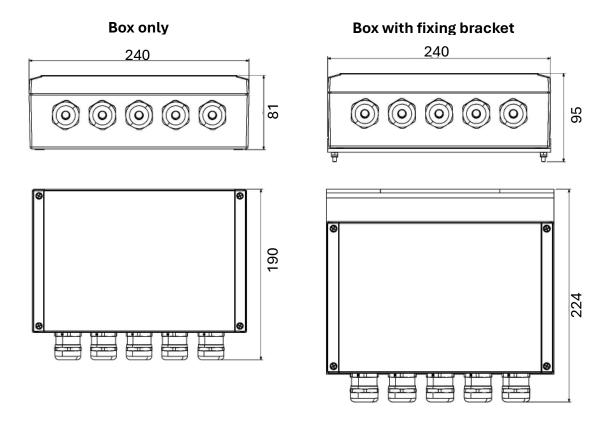
The enclosure is assembled using the four 4.2 mm diameter holes. OBSTA recommends using M4x16 screws with lock nuts.
