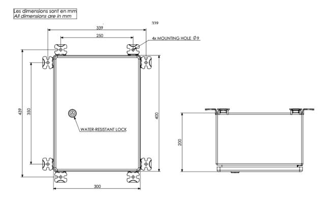
The power supply cabinet (P/N-113797U) is a system available with the OFI-360 not integrated and in 240 Vac version only:
