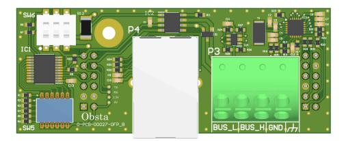
If the Ethernet/CAN pcb module is connected, the command card is able to manage CAN communication, with light status reporting, command processing, flash and D/T/N synchronization.
