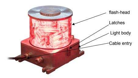
The flash-head includes 6 optics and 6 led strips that ensure the light output of the light. Each flash-head do have 2 independent led circuits.
