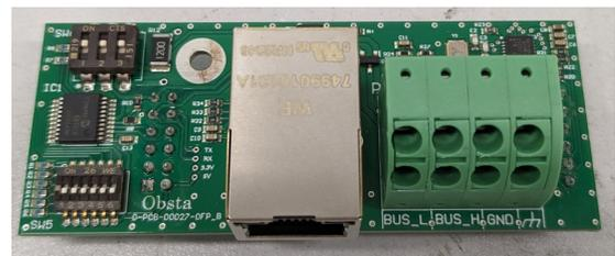
Figure 4: PCBa OFP MI CAN Extension Card
