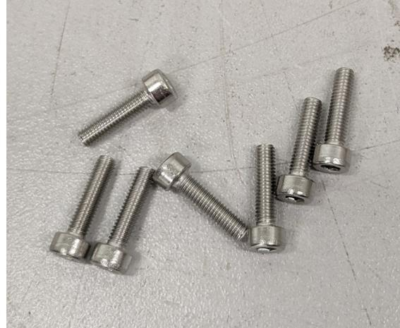
Figure 1: VIS CHC M3X12 INOX A4
