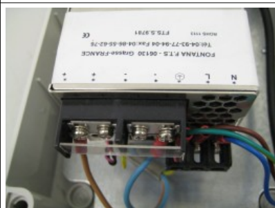
9. Wiring of the 230VAC cable inside the AC → DC power supply
