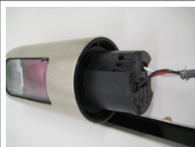
4. Wiring of the 3x1,5mm 2 cable on the 24Vdc photocell
