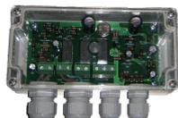
Control 1 or 2 NAVILITE HI 113930 or 113935 either with an active redundancy (one main lamp and one back-up lamp switched on in case of failure of the main lamp)
